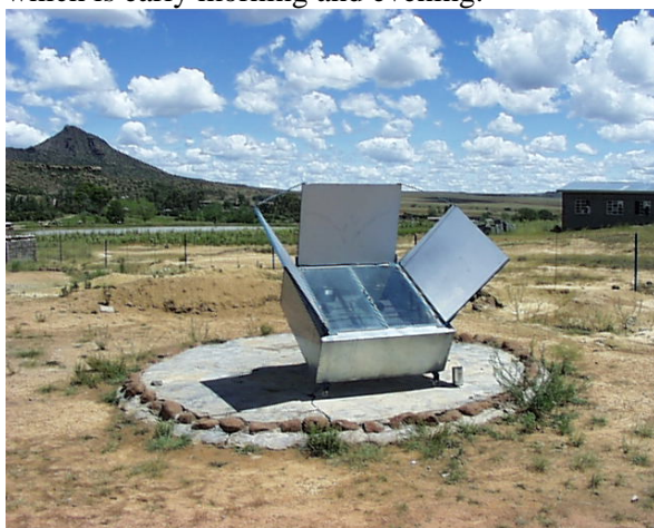
A solar cooker at the Taung Trades Training Centre, near Mochale's Hoek, self constructed and used for preparing meals at neighbouring school.
